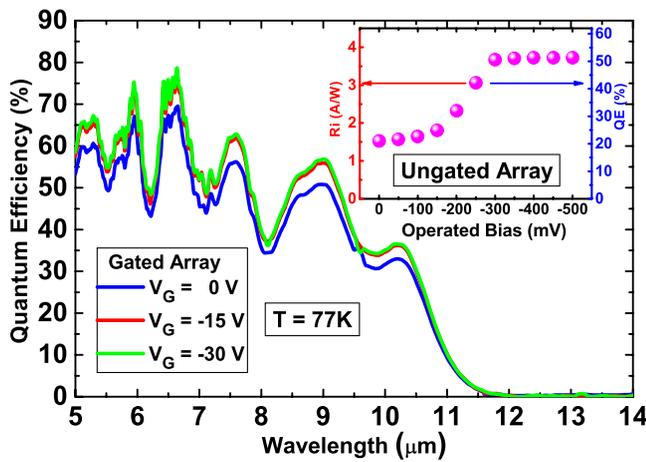
FIG. 2. Saturated spectral quantum efficiency at  $V_{op} = -300$  mV and at different  $V_G$  values in  $Y_2O_3$  passivated GDs. Inset: Peak responsivity (at  $9 \mu m$ ) and the quantum efficiency at peak responsivity of the UGDs at different  $V_{op}$  values.
