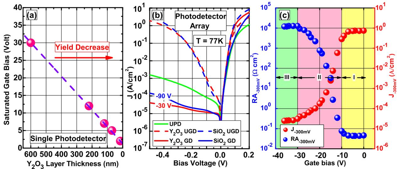
FIG. 1. (a) Correlation between saturated gate bias and  $\text{Y}_2\text{O}_3$  passivation layer thickness of samples A2–A6. (b) Comparison of dark current density of the UPD and UGD with  $\text{SiO}_2$  and  $\text{Y}_2\text{O}_3$  passivation, and GD with  $\text{SiO}_2$  and  $\text{Y}_2\text{O}_3$  passivation. (c) The dependence of reverse dark current density and differential resistance area product on gate bias in  $\text{Y}_2\text{O}_3$  passivated GDs at  $V_{op} = -300$  mV.
