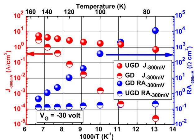
FIG. 3. The evolution of the  $J_{-300mV}$  and  $RA_{-300mV}$  of  $Y_2O_3$  passivated GDs and UGDs at  $V_G = -30$  V with temperature.
