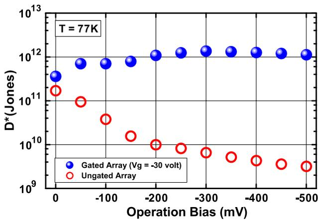
FIG. 4. Specific detectivity of  $\text{Y}_2\text{O}_3$  passivated UGD array and GD array at  $V_G = -30$  V calculated at different  $V_{op}$  values.
