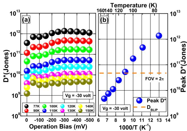
FIG. 5. (a) The evolution of the detectivity of  $\text{Y}_2\text{O}_3$  passivated gated diode array with temperature at  $V_G = -30$  V and different  $V_{op}$ . (b) The evolution of the peak detectivity of  $\text{Y}_2\text{O}_3$  passivated gated diode array with temperature. The peak detectivity crosses the BLIP line at 110 K.
